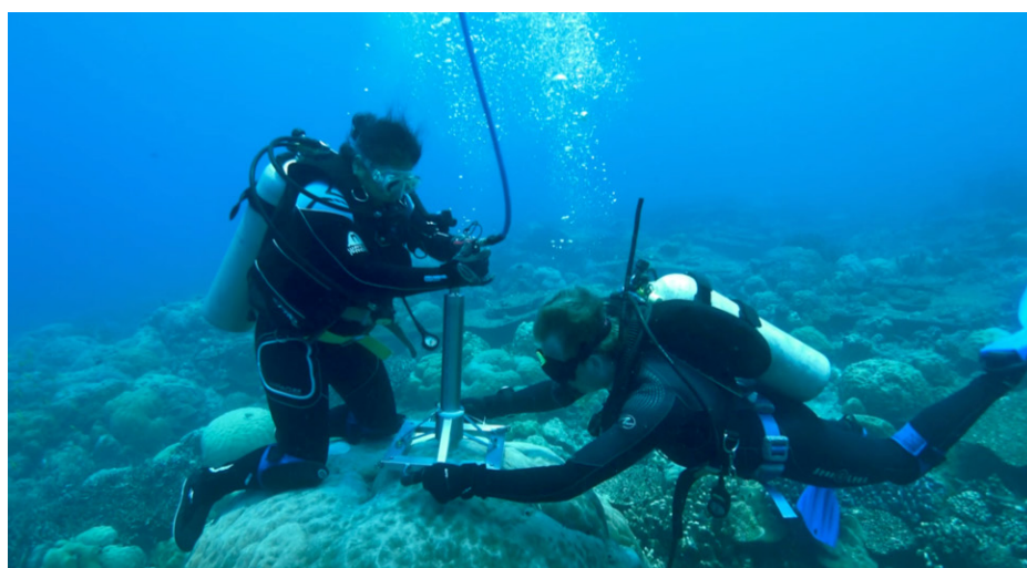
Figure 1: Extracting a core from a coral colony at Christmas Island (Indian Ocean). Photo credit: Jason Turl.
